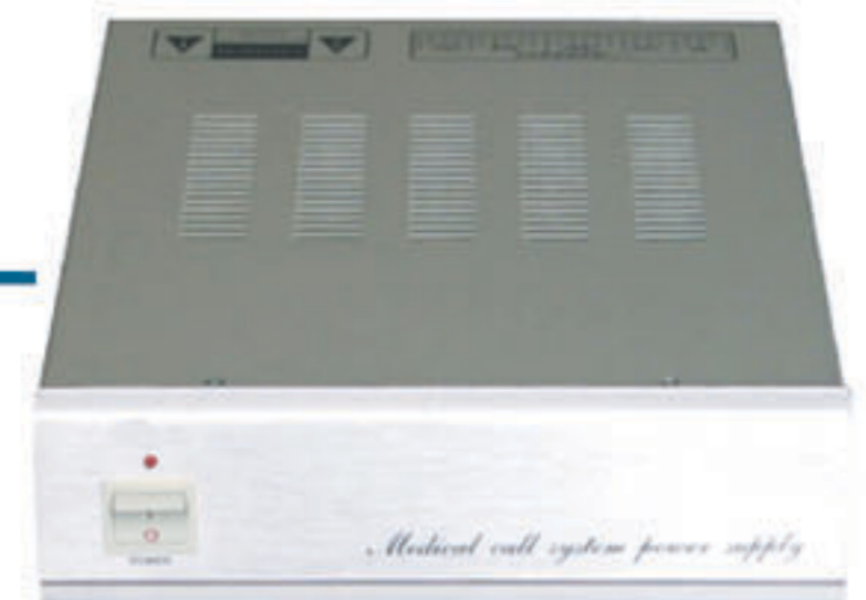
Dimension: 215 X 285 X 70MM (L X W X H) Installation illustration: Install at nurse working counter, need to setup/allocate a dedicated AC 220V power supply socket, the socket should design for single-circuit, with the condition needing approval prior to the inclusion into the hospital UPS system.
